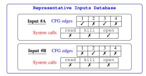
To establish which of **Input #A** and **Input #B** has the closest combination of CFG edges compared to **Input #1**, we compute the Hamming distance [42] between the CFG edge vectors and consider the one for which the distance is the smallest. In this case, **Input #A** is retrieved, as its coverage w.r.t. **Input #1** differs only by two edges, against three for **Input #B**:
